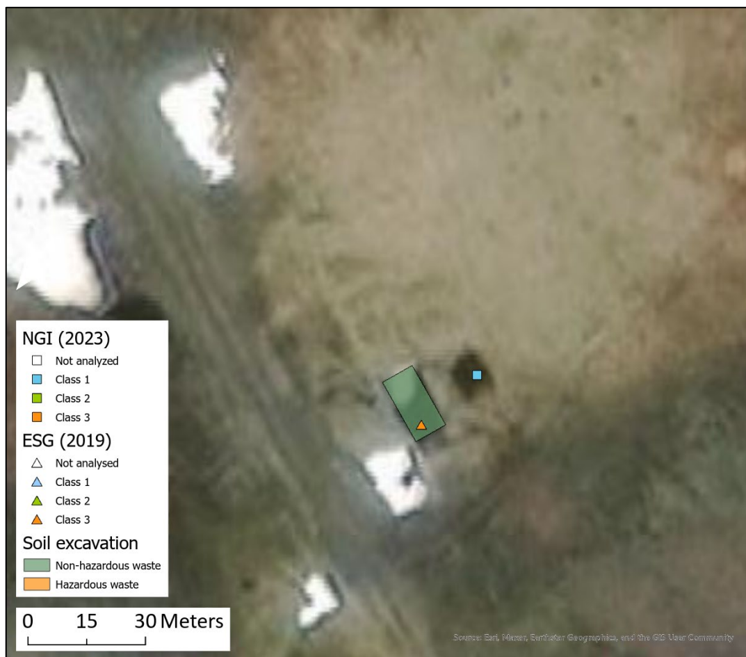
Figure 3-5 Excavation plan for the small pond in the Catchment Area.
