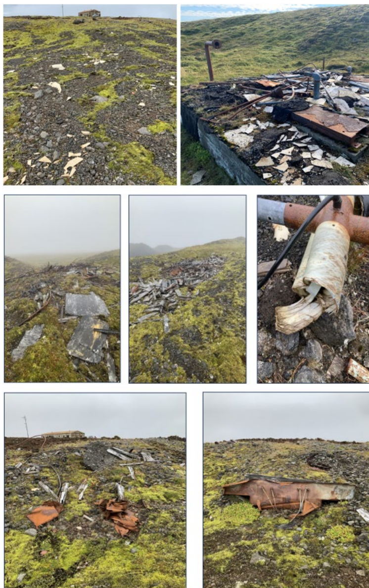
Figure 3-6 Examples of pale-yellow fragments of asbestos-containing building materials (top), wood debris and wires (center) and scrap metal, wires and wood (bottom) present on Heidarfjall.
